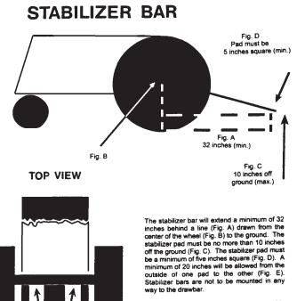
NOTE: The stabilizer bar system must be able to support the weight of the tractor in the heaviest class pulled. Jacking up the pads so tractor is completely off the ground is a good test.
