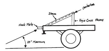
This is one example of a 25 degree hitch angle. Your hitch construciton does not have to look exactly like this one.
